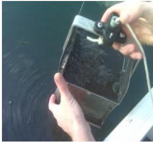
A sampler for lake sediment sampling
